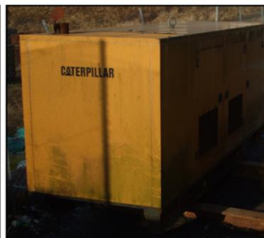
Caterpillar 3306B generator, 200kW, 400 v (3 phase), 250 KVA, manufactured 2003 with approximately 11249 working hours
