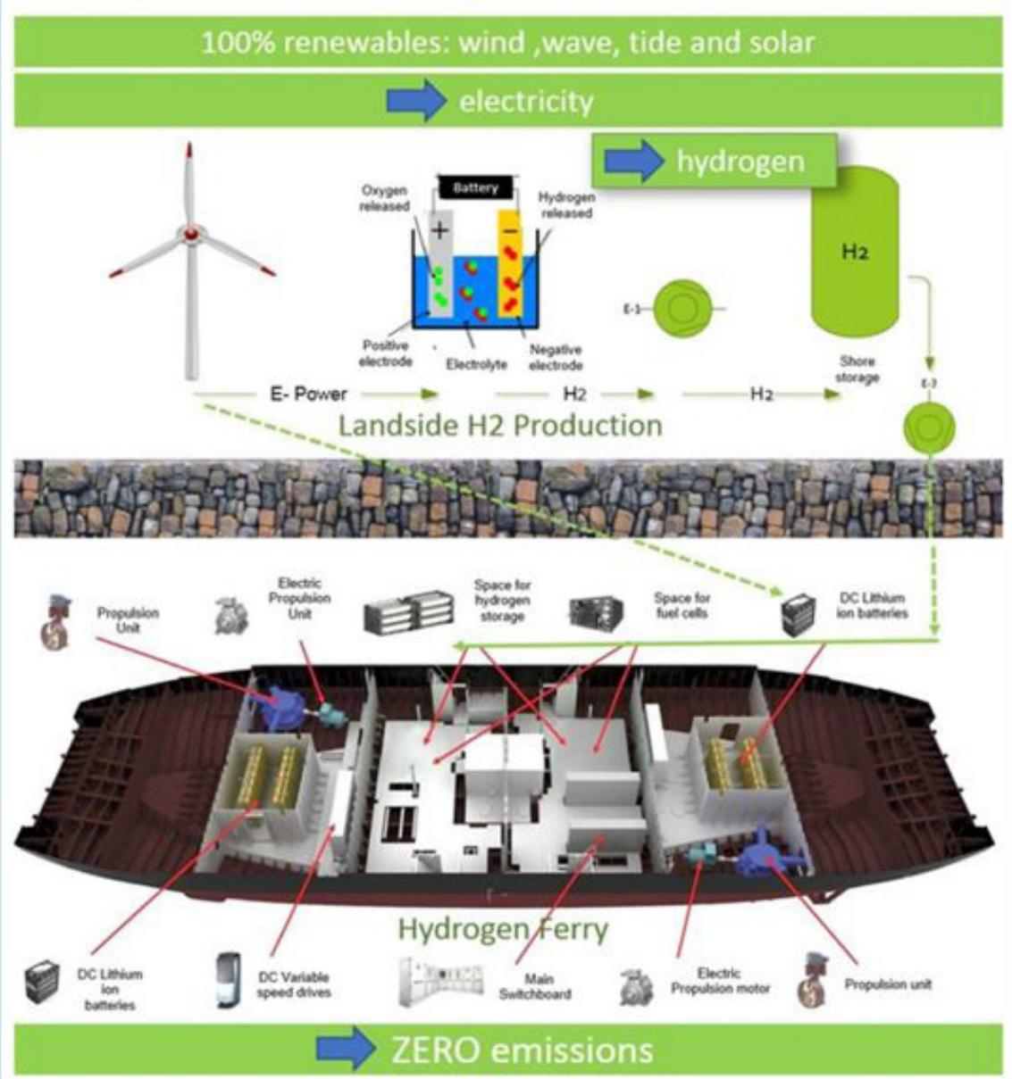
HySeas III is looking to design, test and build a hydrogen fuel cell ferry to service the Kirkwall to Shapinsay ferry route. According to preliminary results from the HySeas III project the Fuel Cell & Battery Kirkwall to Shapinsay ferry could enable a reduction up to 90% of the Global Warming Potential from cradle to the end of life with regards to a conventional Diesel ship when both hydrogen and electricity are produced by wind turbines.
