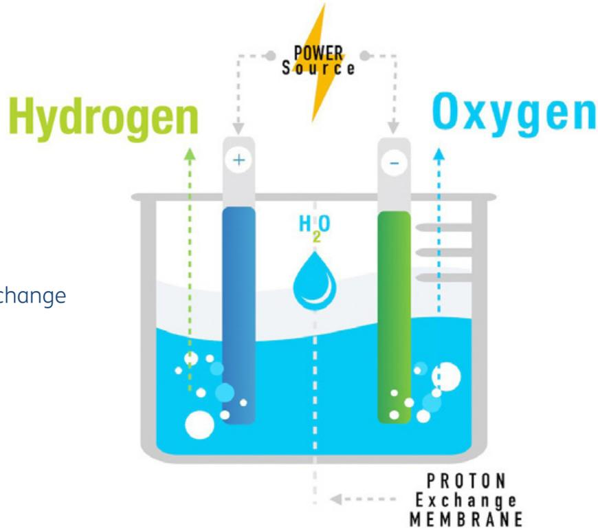
Figure 3: Proton exchange membrane (PEM) electrolyses.
